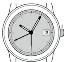
The crown is unscrewed. To wind the watch manually, turn the crown clockwise; the other direction is inactive. When first activating the watch or after a stoppage, turn it through at least 25 revolutions to ensure it is partially wound.
